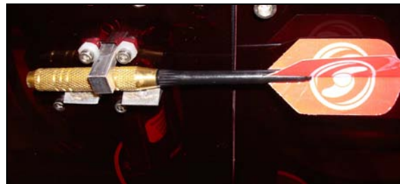
One of Triton's marker droppers holding a CUAUV customized dart.
