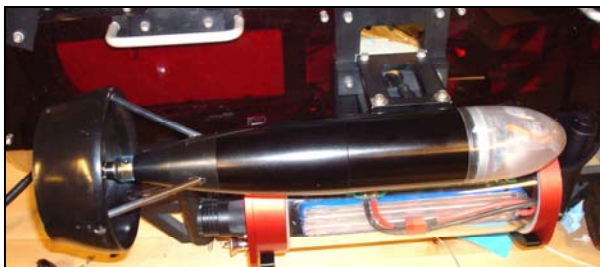
VideoRay GTO Thruster mounted to Triton.
