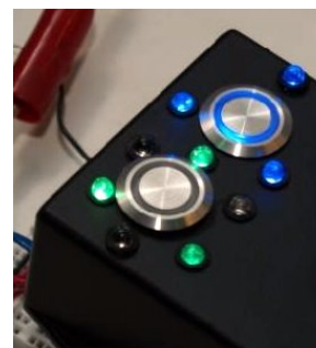
Figure 15: Switchbox with motors unkilld and mission started
